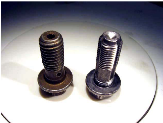
Cross drilled flow bolt on left, new design on right
