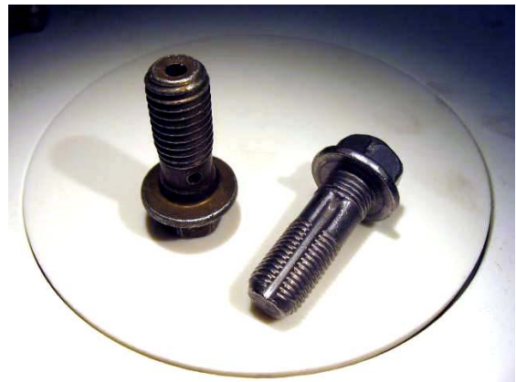
Cross drilled flow bolt on left, new design on right
